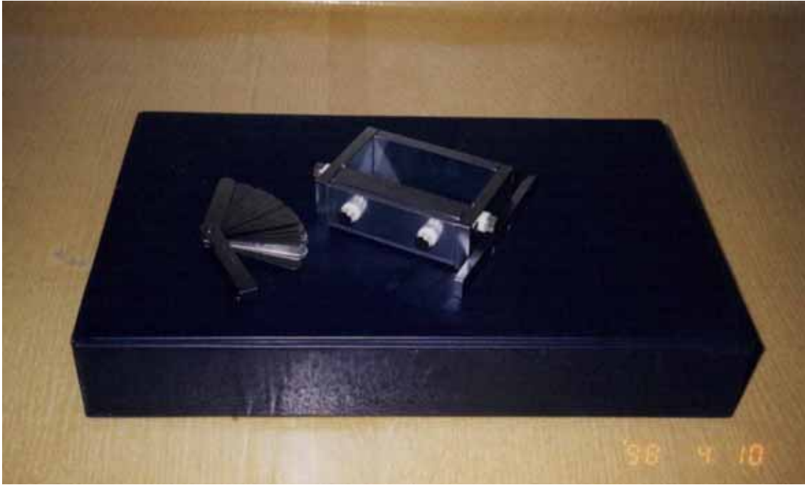
MANUAL (HAND) TAPE CASTING JIG (Model MTC-01A and THICKNESS GAUGE
